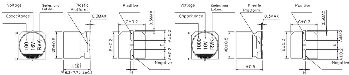
\*1. Voltage mark for 6.3V is [6V]      6.3V的产品标识为 [6V]
